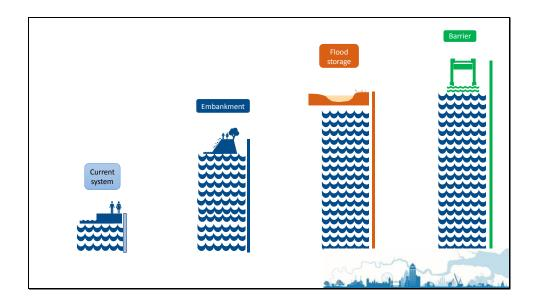
In this example, the current system protects us against a modest increase in sea level. Beyond that, there are 3 options for flood defences that we could build. A flood embankment, a tidal flood storage area, and a tidal barrier. Each would protect us across a range of sea levels, indicated here by the coloured bars, up to a certain threshold of sea level rise.
