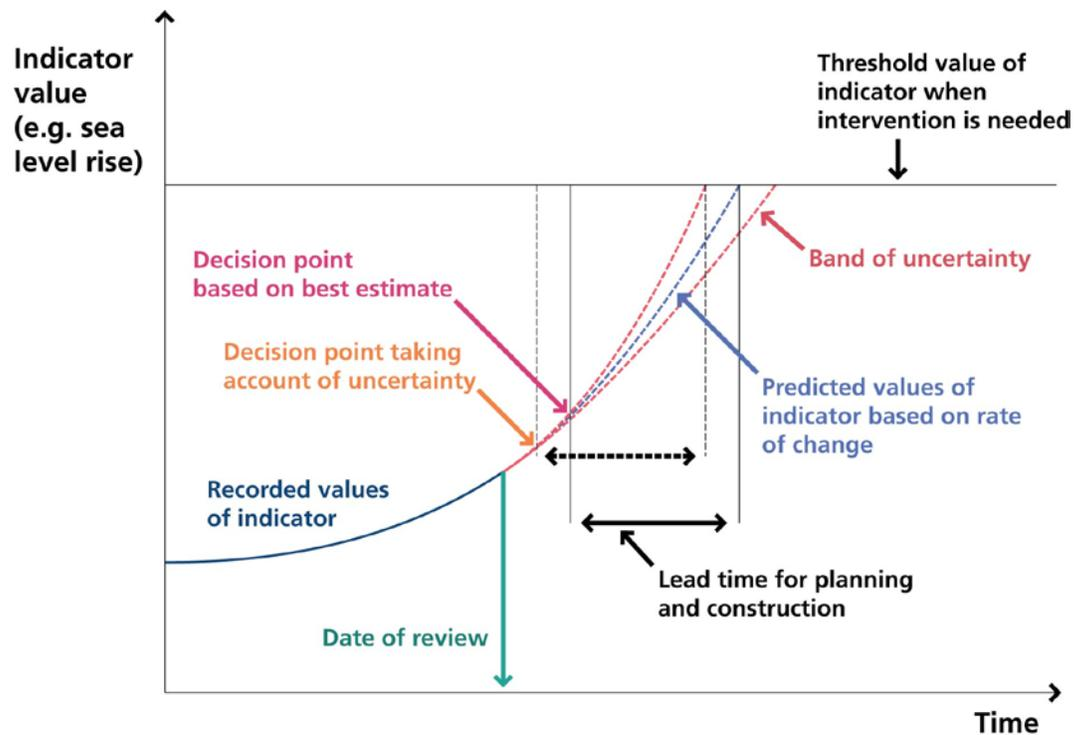
Figure 3. Schematic diagram of the thresholds, lead times and decision points approach from TE2100
