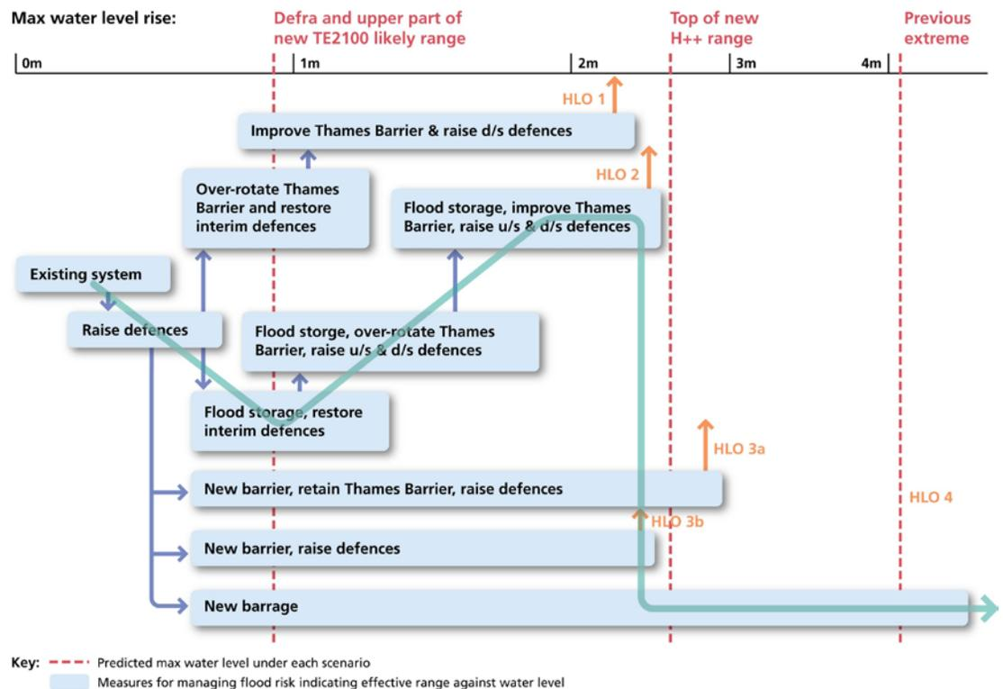
**Figure 2. High-level adaptation options and pathways developed by TE2100 (on the y-axis) shown relative to threshold levels increase in extreme water level (on the x-axis). The blue line illustrates a possible ‘route’ where a decision maker would initially follow HLO 2 then switch to HLO4 if sea level was found to increase faster than predicted.**
